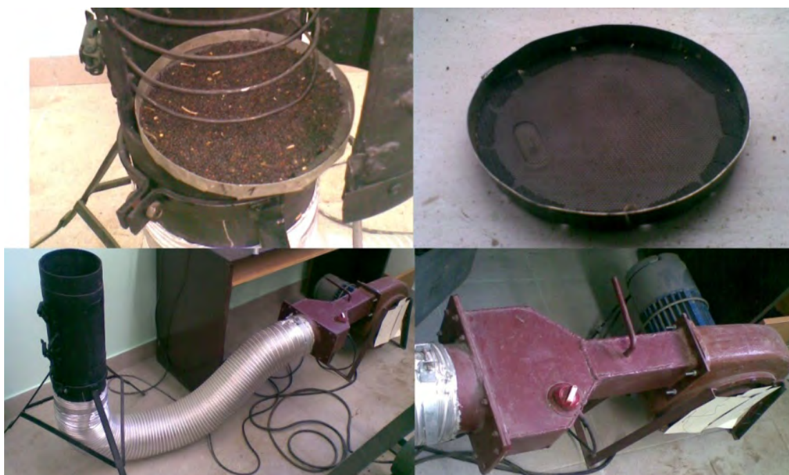
Figure 3 – Installation for studying the process of drying rapeseeds
